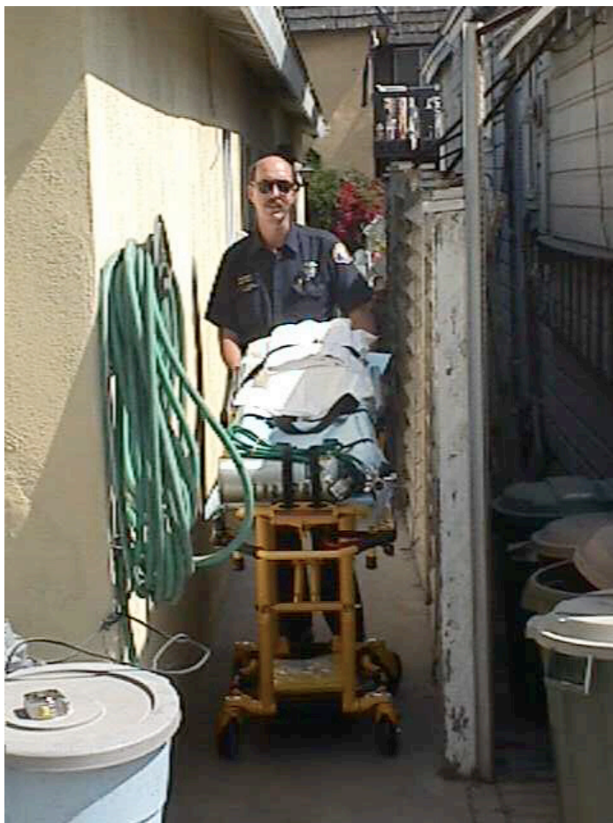
Figure 5-6: Newport Beach Fire Department personnel illustrating the difficulty of maneuvering emergency equipment and victims through the 3-foot allowable building setback, especially if non-structural additions project into this area. Dumpsters and other things stored in this area can also make access to the back of a residence difficult, if not impossible. Residents should maintain this area free of obstructions.
