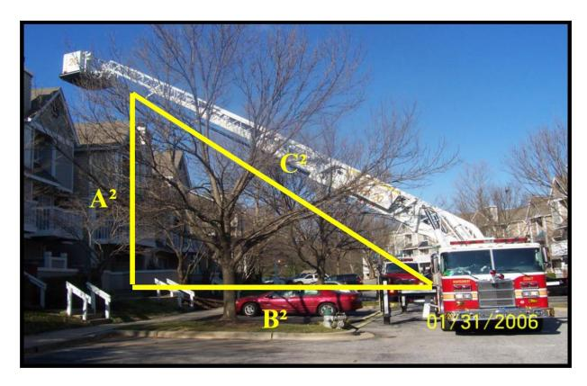
In this illustration, "A" equals the height of the building (use 12 feet per floor for commercial and multi-family structures), "B' equals the distance from the building to the turntable and "C" is the required distance to reach the building.
