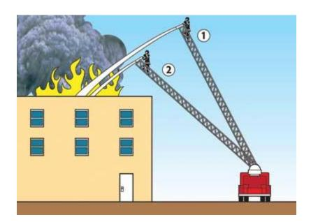
Aerial positioning is dependent on many factors such as access, type of structure, primary objectives, hazards, obstructions and most importantly the reach of the aerial ladder. This determination of positioning will be subject to a case by case basis but at a minimum the Quint or (ladder truck) has to minimum of 15 feet and a maximum of 35 feet from the building. This gives the ladder the greatest load capability when maintained between 40 to 75 degress.
