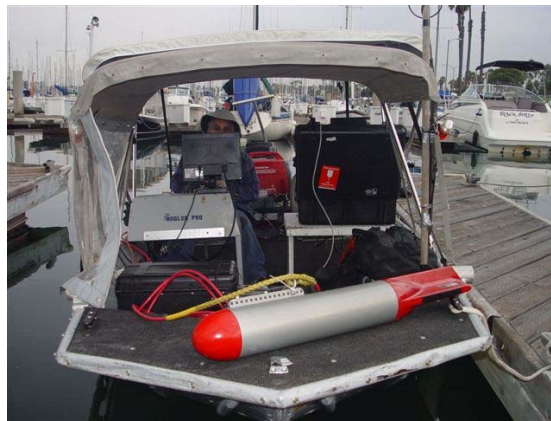
Photograph 8. Imagenex 881 Sportskan Sidescan Sonar Towfish
