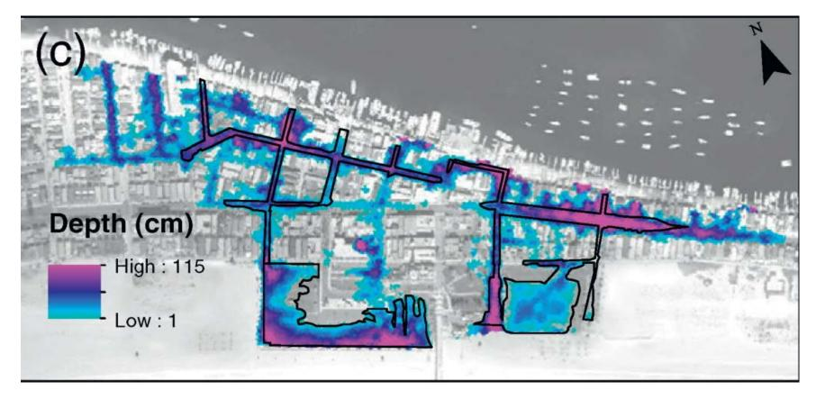
**Figure 4.** Observed flood extent (solid black line) vs. flood extent predicted using the HR and BreZo modeling methodology, for the August 2011 wave overtopping event at Newport Beach. Extracted from Gallien et al. (2014).
