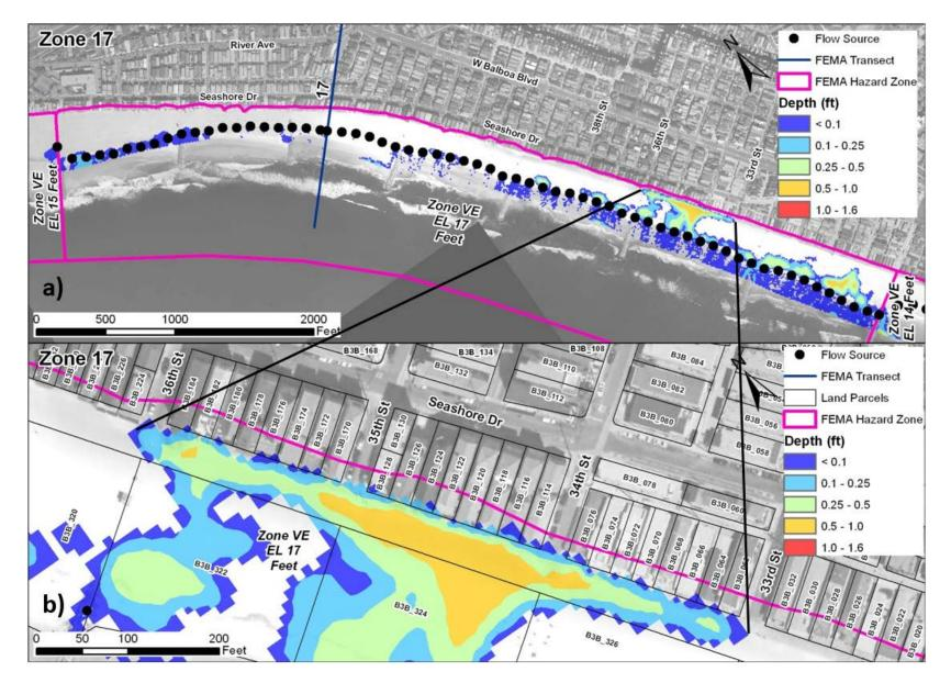
Figure 6. Wave overtopping at Zone 17. a) Overview of shoreline reach and b) magnified view between 33rd and 36th St.
