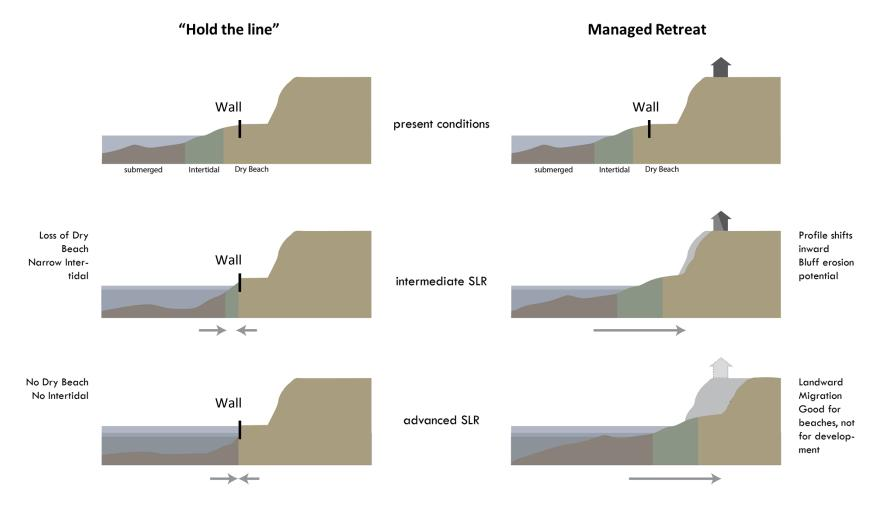
Figure 7-1: Illustration of Hold-the-Line Versus Managed Retreat Approaches
