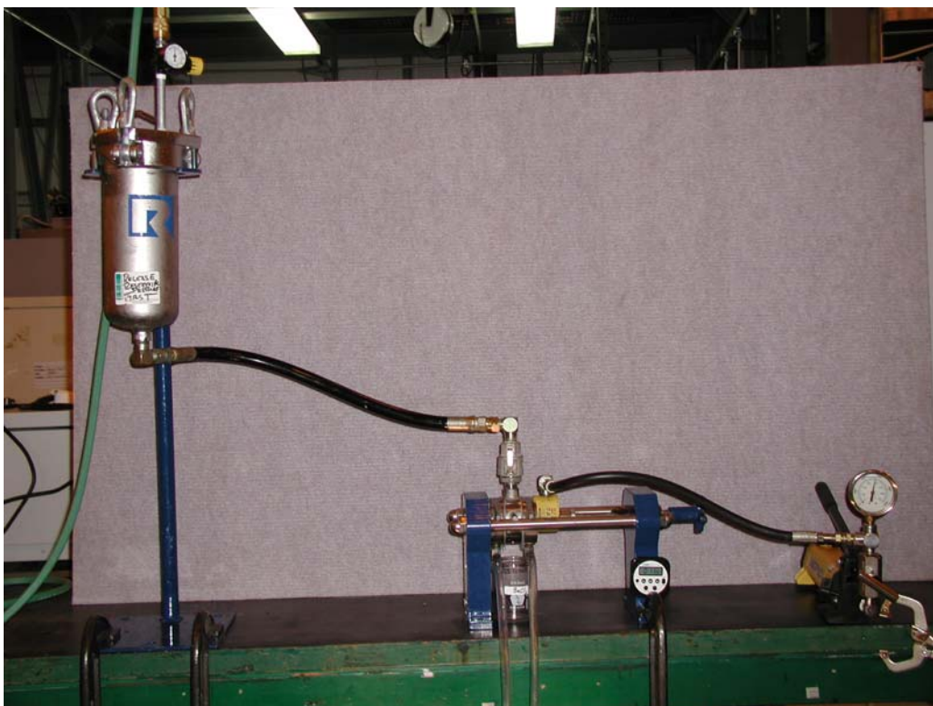
Figure A-1 US Filter 7.62 cm Bench Top Press (Model 75N-1-MYHS), Reservoir, Chamber and Hydraulic Ram
