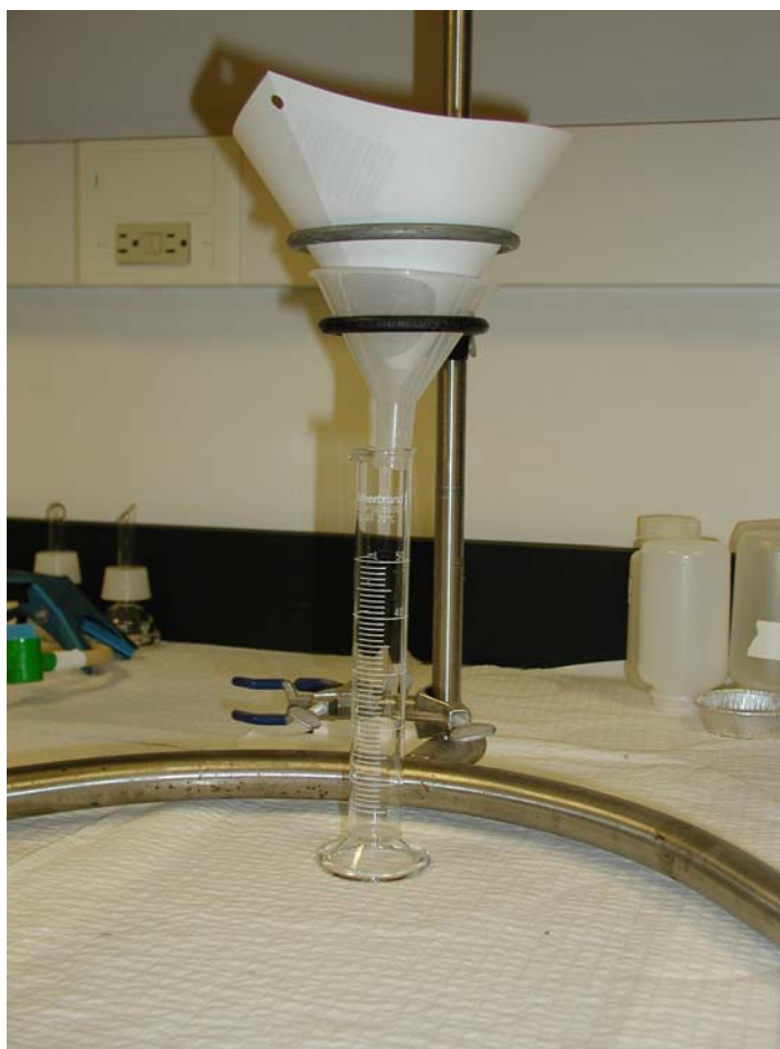
Figure A-3 Paint Filter Test Setup
