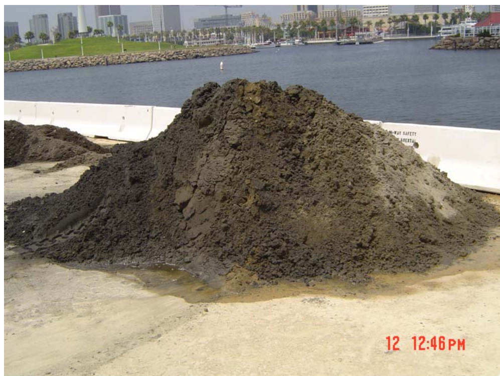
Figure C-9 Field Pilot Study – Washed Sand Output from 10” Hydrocyclone
