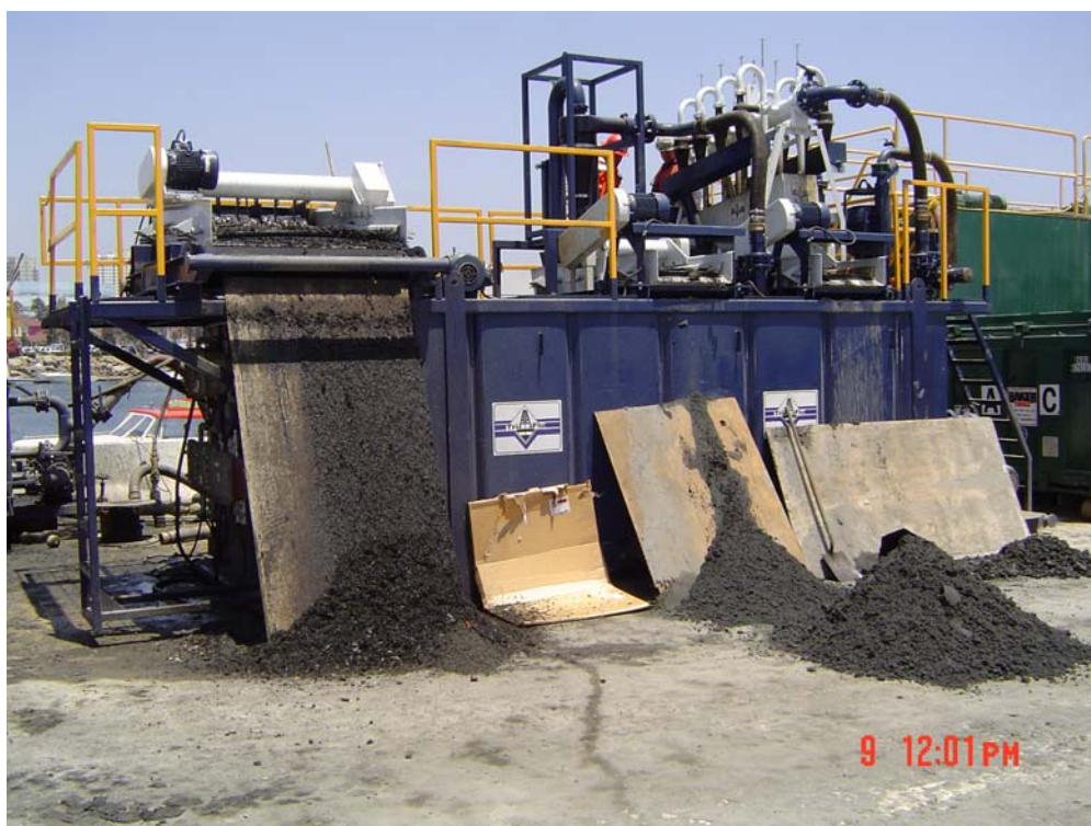
Figure C-7 Field Pilot Study – Hydrocyclone in Operation
