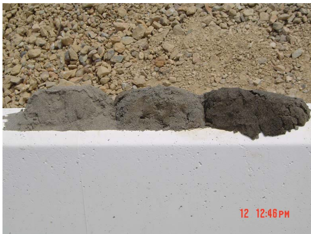
Figure C-10 Washed Sand after 24, 48, and 96 Hour Post Processing (right to left)
