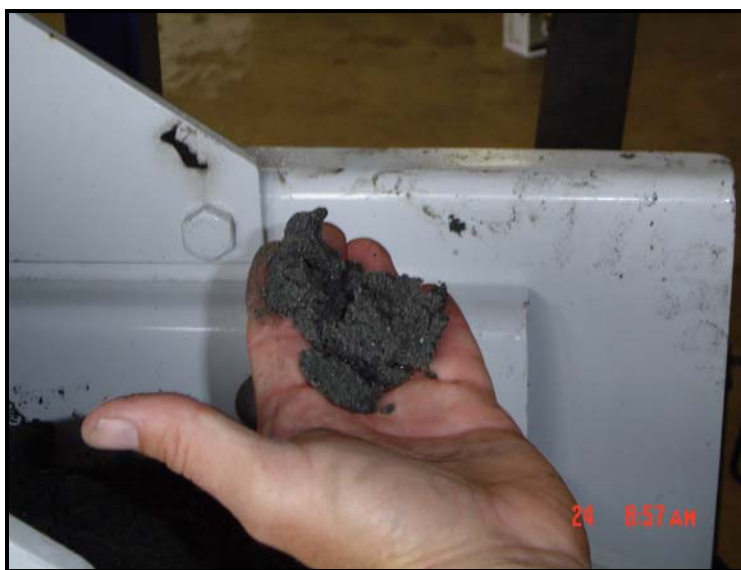
Figure B-4 Sand Material Passing Through the 4” Hydrocyclone
