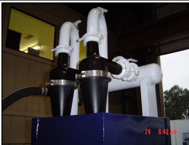
Figure B-2 Tri-Flow International View of 4" Hydrocyclones
