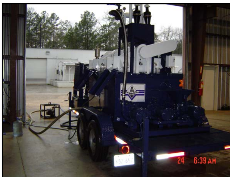
Figure B-1 Tri-Flo International 4" Mobile Hydrocyclone Unit
