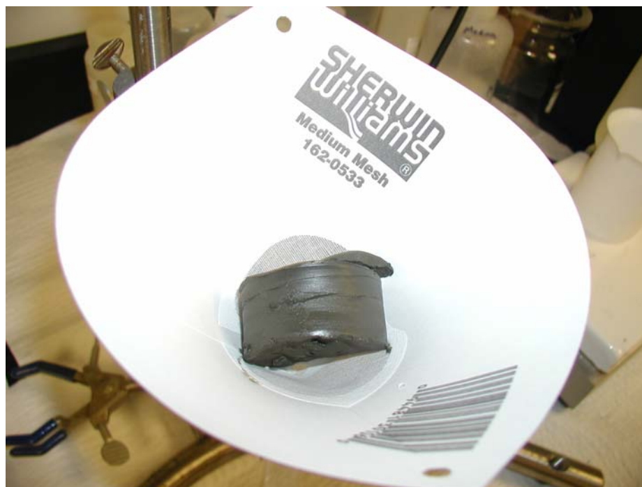
Figure A-11 Paint Filter Test of Dewatered Cake
