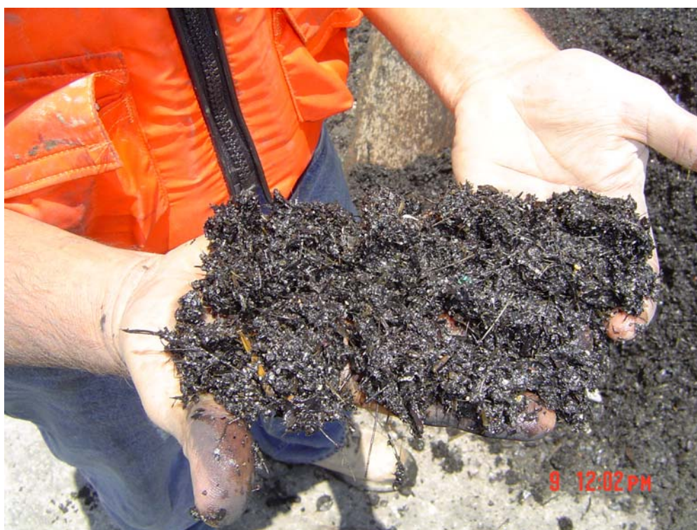
Figure C-8 LARE Debris Removed from Scalper Unit
