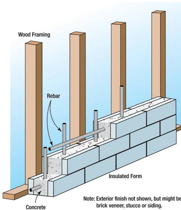
**Figure 6-4. Insulating Concrete Form**
