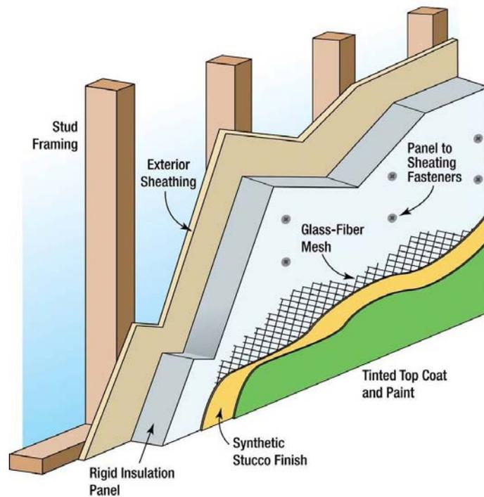
Figure 6-9. Exterior Insulation Finishing System
