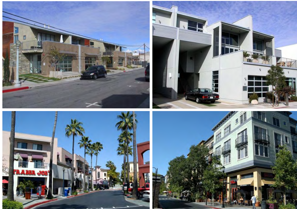
Illustrates mixed-use buildings that integrate ground floor retail and upper floor residential. Modulated building volumes and articulated elevations, separate entries for retail and residential, and orientation of the building to pedestrian-oriented streets.
