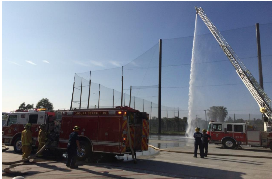
Pictured above: Laguna Beach Engine 1 supplies Newport Truck 62 with water for a “water tower operation.”
