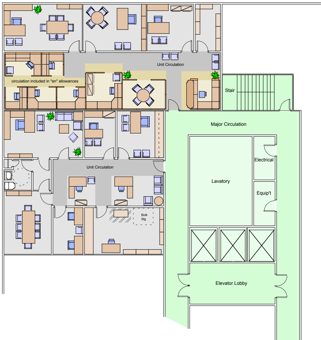
Illustration Showing Gross SF Areas of Building and Showing Hypothetical Office Suites
