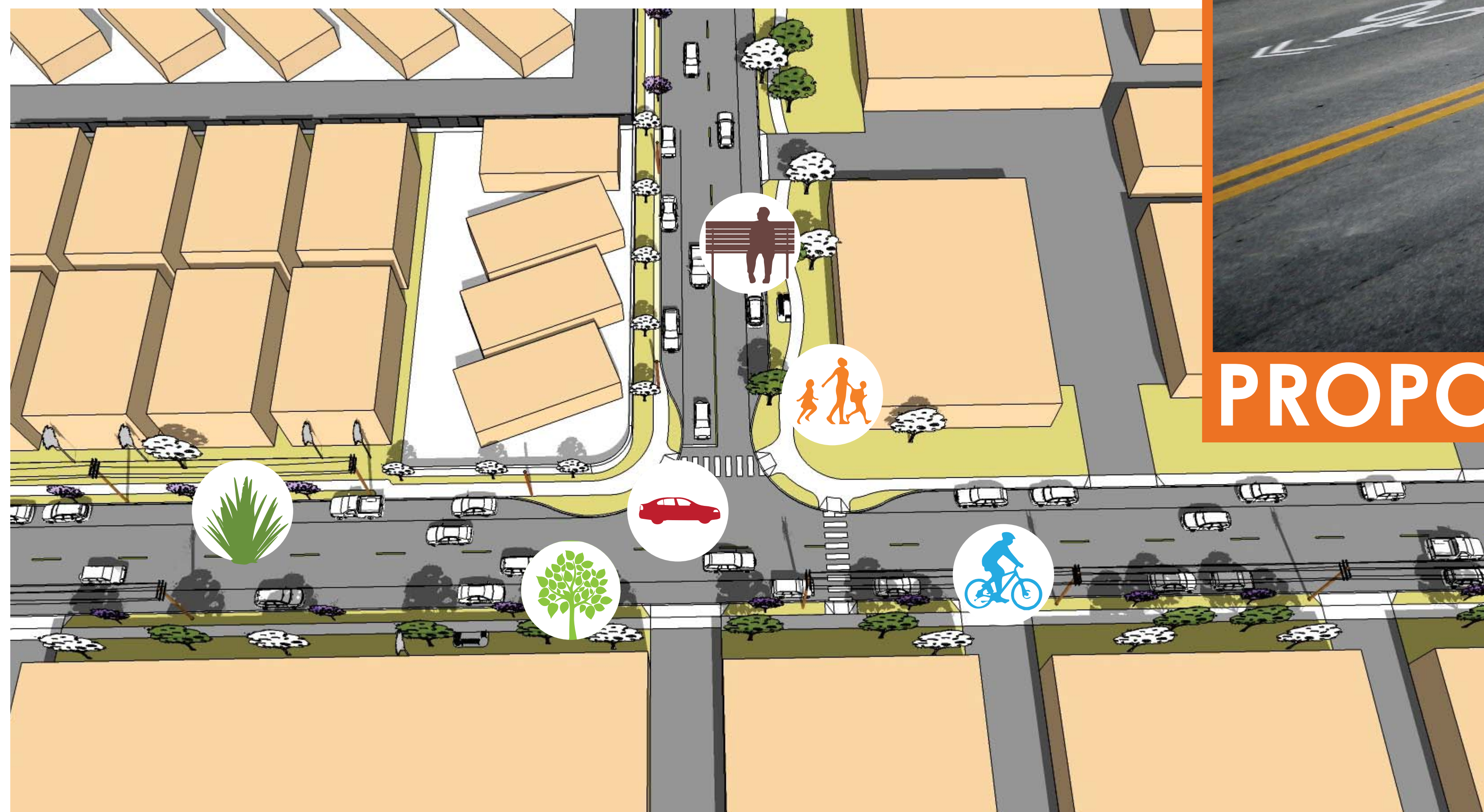
BULBOUT ON MONROVIA AVENUE
