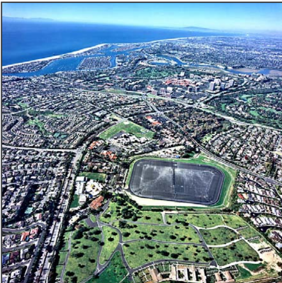
During this past year, the Big Canyon Reservoir Cover and Disinfection Project was completed. The cover was installed on the reservoir to improve the water quality and protect the City's drinking water source. The area of the cover is approximately 23 acre feet.
