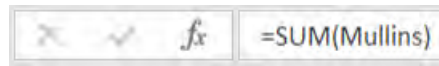
Figure 1–6: Named cells and ranges make it easy to identify the purpose of formulas and to enter cell and range references accurately.
