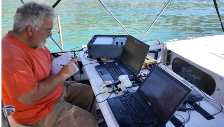
Photograph 9. Hypack Navigation Software Used by Nearshore and Wetland Surveys for Steering Vessel Along Tracklines. Steering Position Was Relayed Via Monitor to Skipper.
