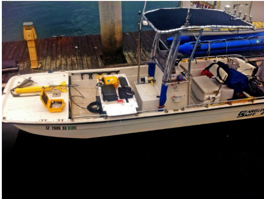
Photograph 7. CRM's Research Vessel Showing Set Up for Sidescan Sonar Surveying
