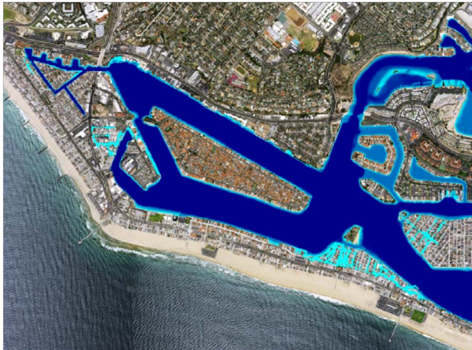
(b) Predicted flooding extent - HEC-RAS Model Validation results
