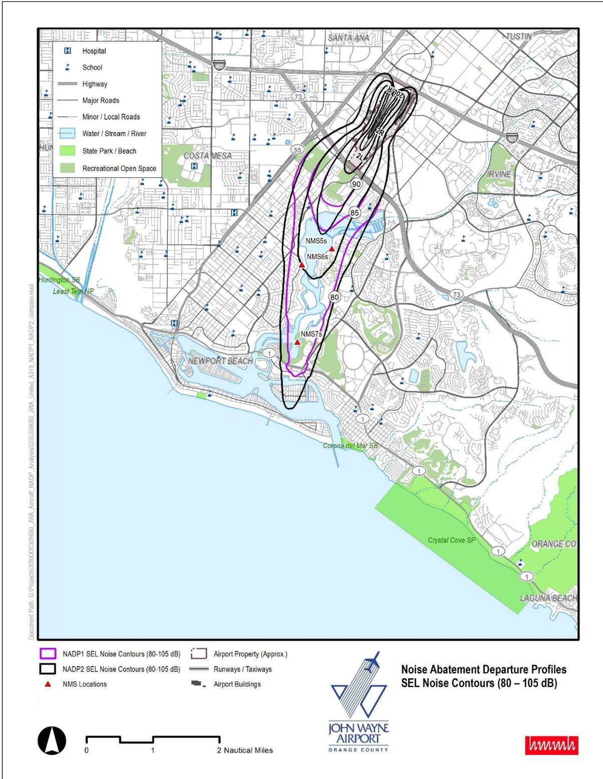
Figure 7. Airline D Airbus A319 NADP SEL Contours
