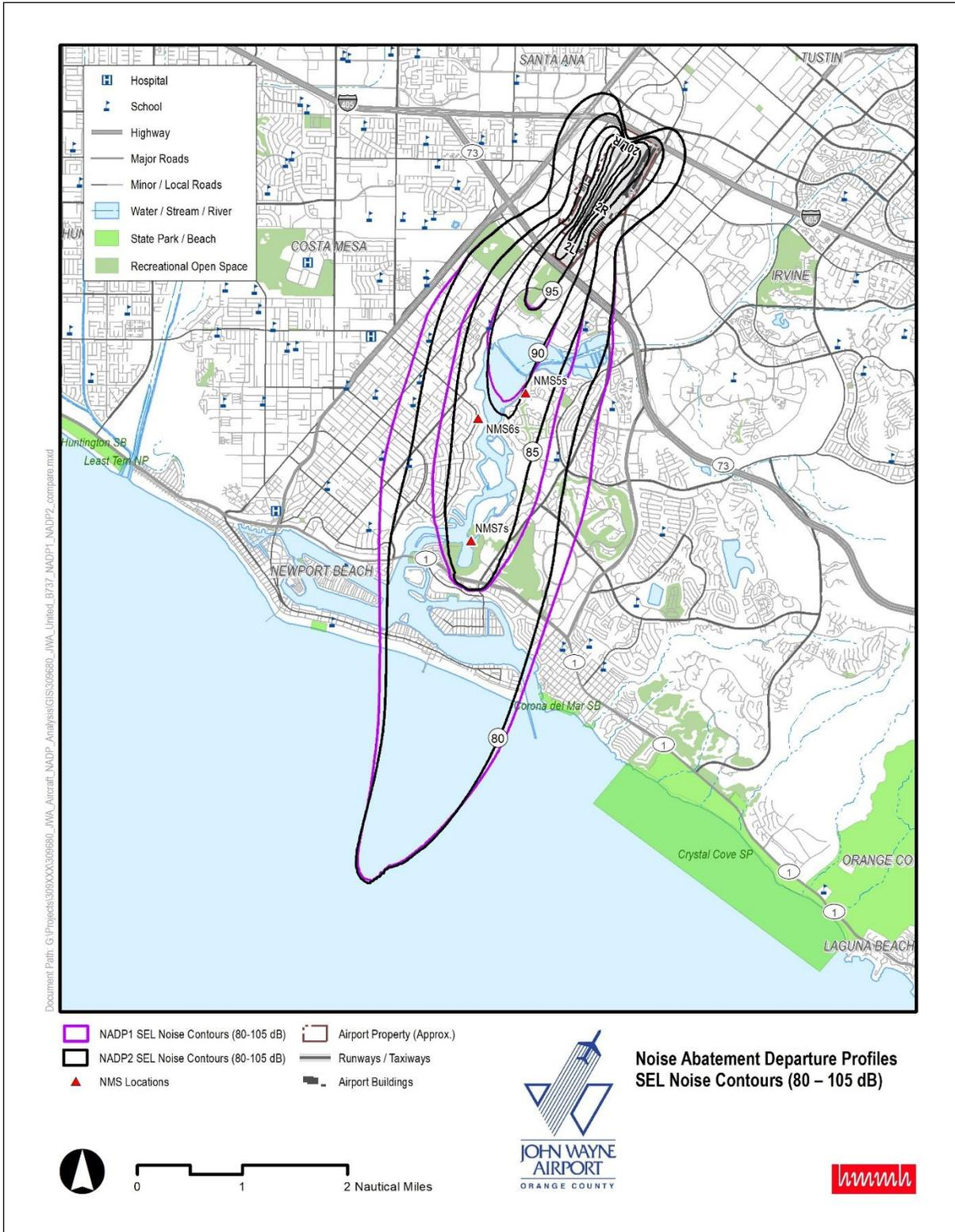
Figure 5. Airline D Boeing 737-700 NADP SEL Contours
