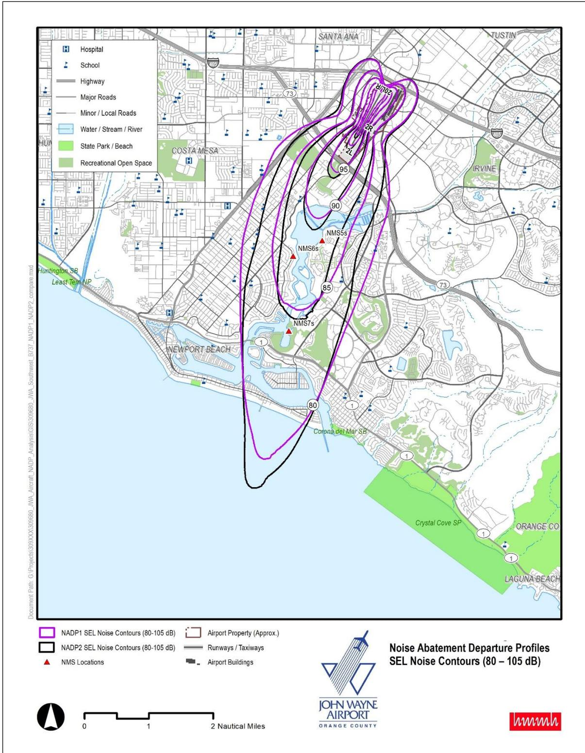
Figure 3. Airline C Boeing 737-700 NADP SEL Contours
