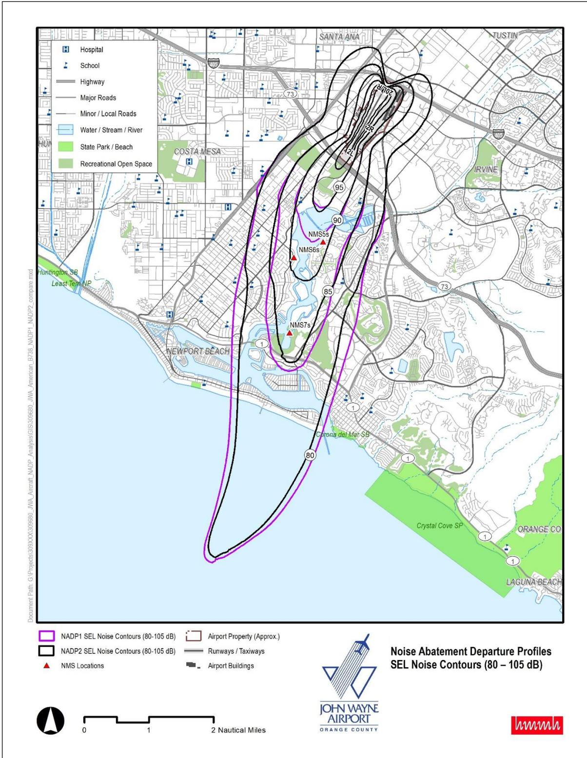
Figure 2. Airline B Boeing 737-800 NADP SEL Contours
