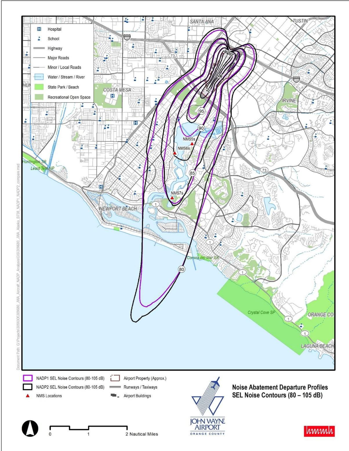
Figure 1. Airline A Boeing 737-800 NADP SEL Contours
