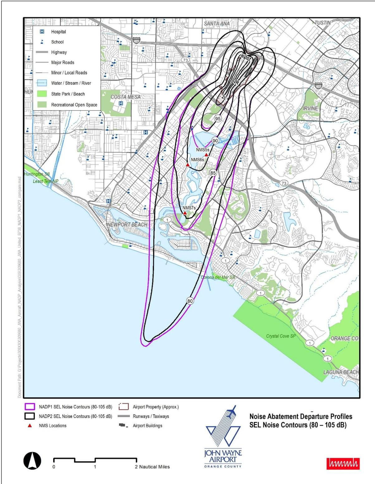
Figure 6. Airline D Boeing 737-800 NADP SEL Contours
