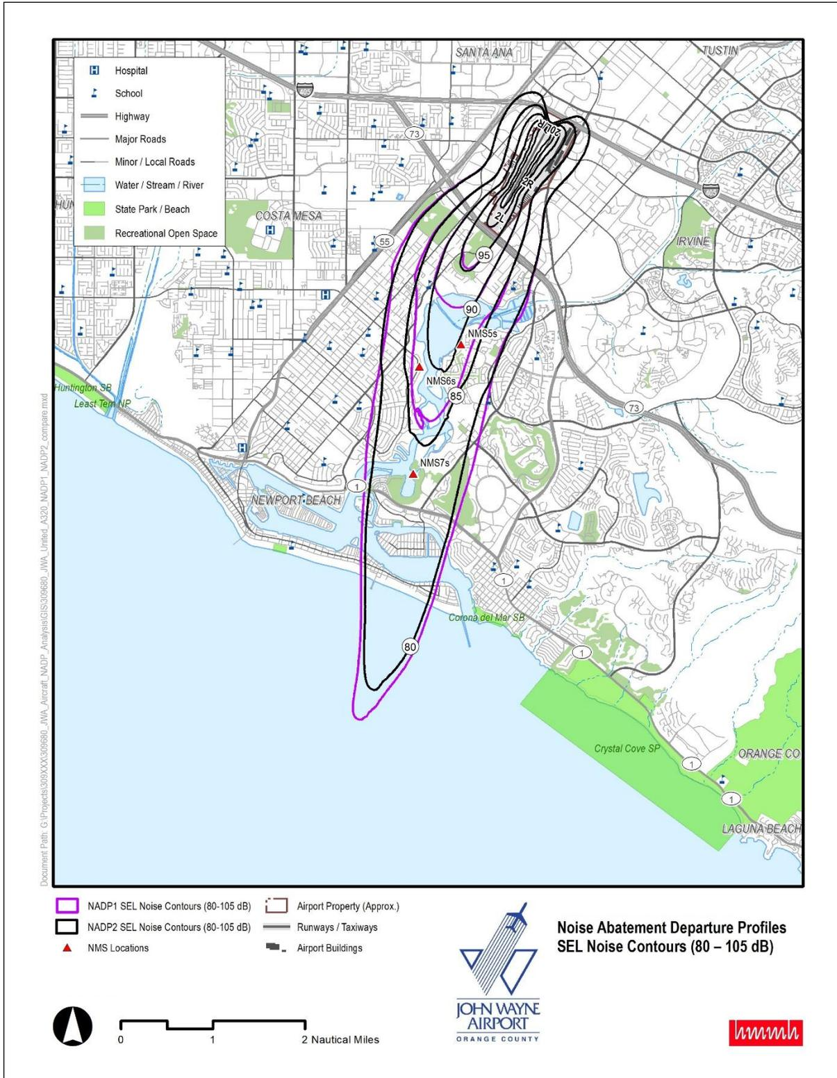
Figure 8. Airline D Airbus A320 NADP SEL Contours
