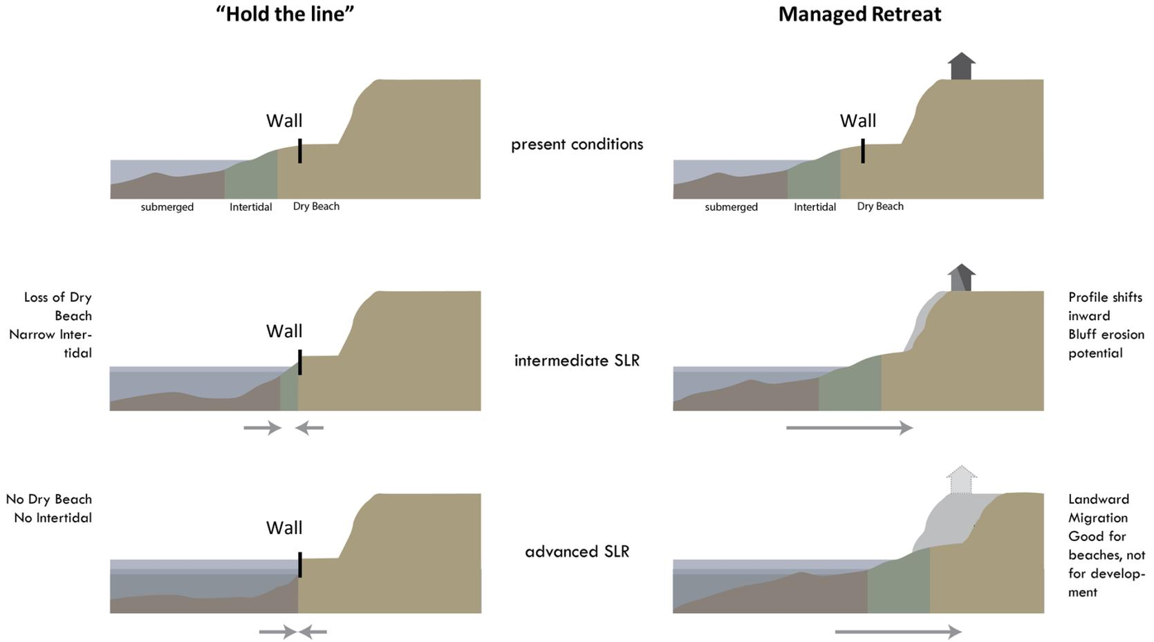
Figure 7-1: Illustration of Hold-the-Line Versus Managed Retreat Approaches
