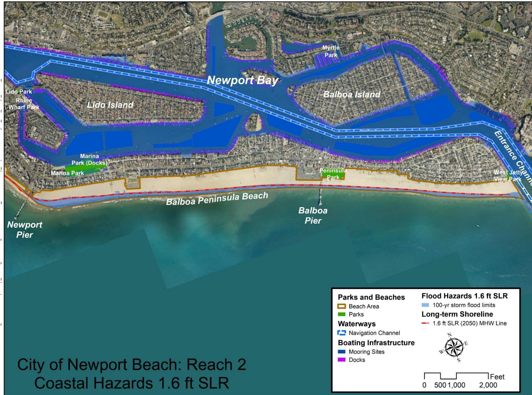
Figure 5-8: Parks, Beaches, Boating Infrastructure, and Submerged Tidelands Assets with 1.6 Feet SLR (Year 2050) Hazards – Reach 2
