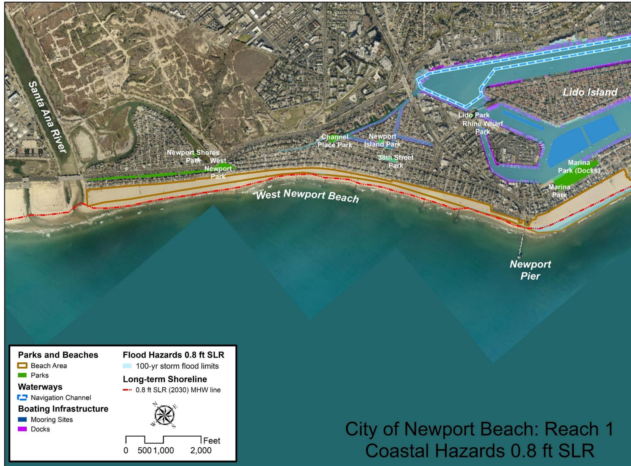
Figure 5-3: Parks, Beaches, Boating Infrastructure, and Submerged Tidelands Assets with 0.8 Feet SLR (Year 2030) Hazards – Reach 1
