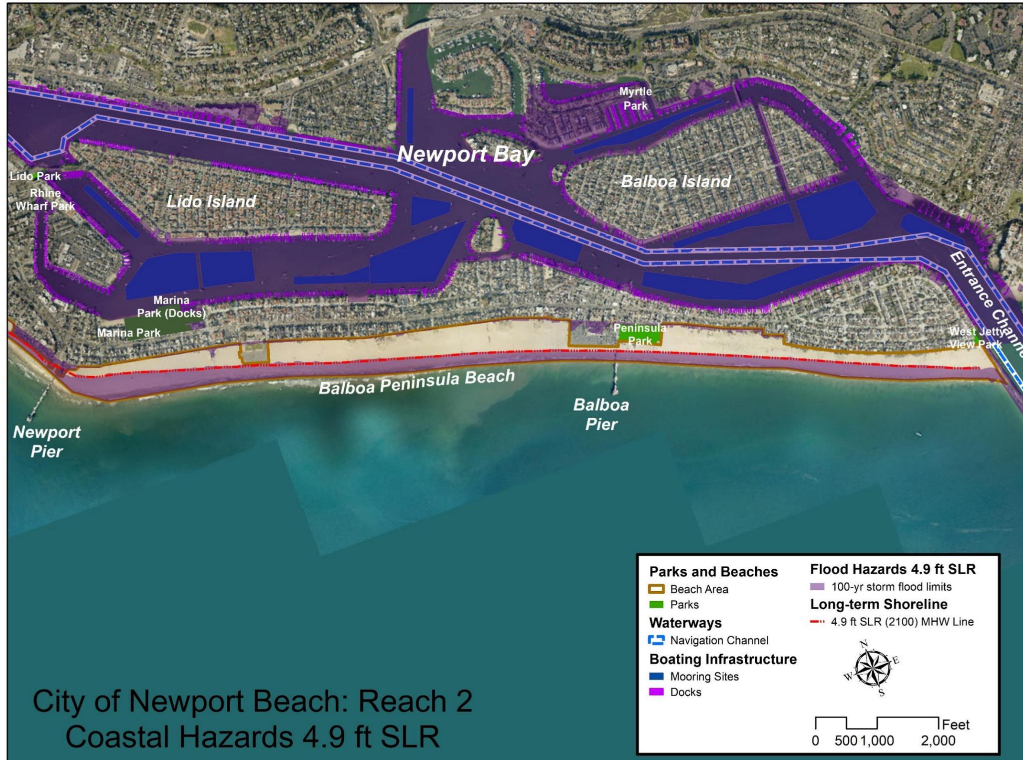
Figure 5-12: Parks, Beaches, Boating Infrastructure, and Submerged Tidelands Assets with 4.9 Feet SLR (Year 2100) Hazards – Reach 2
