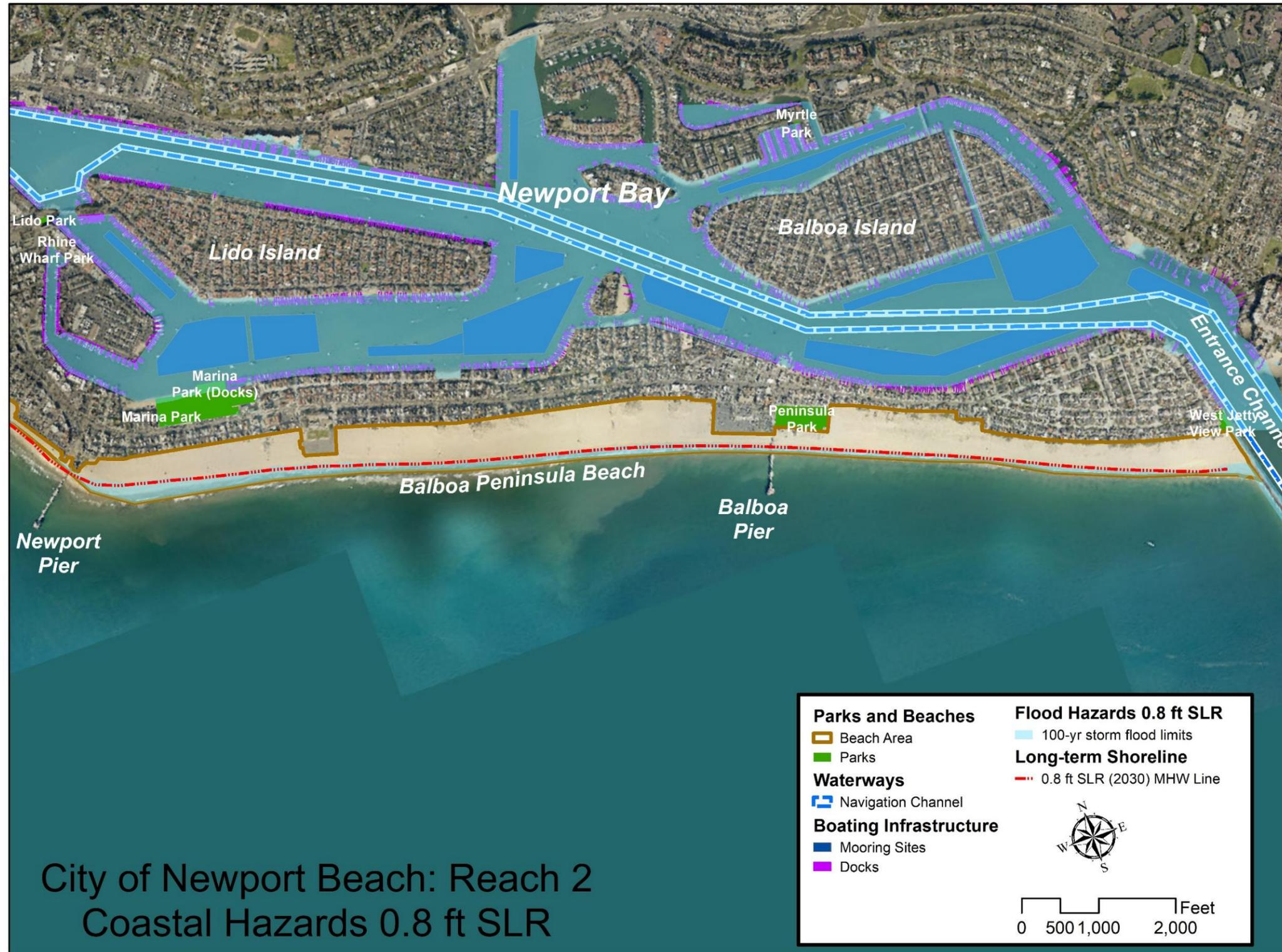
Figure 5-4: Parks, Beaches, Boating Infrastructure, and Submerged Tidelands Assets with 0.8 Feet SLR (Year 2030) Hazards – Reach 2
