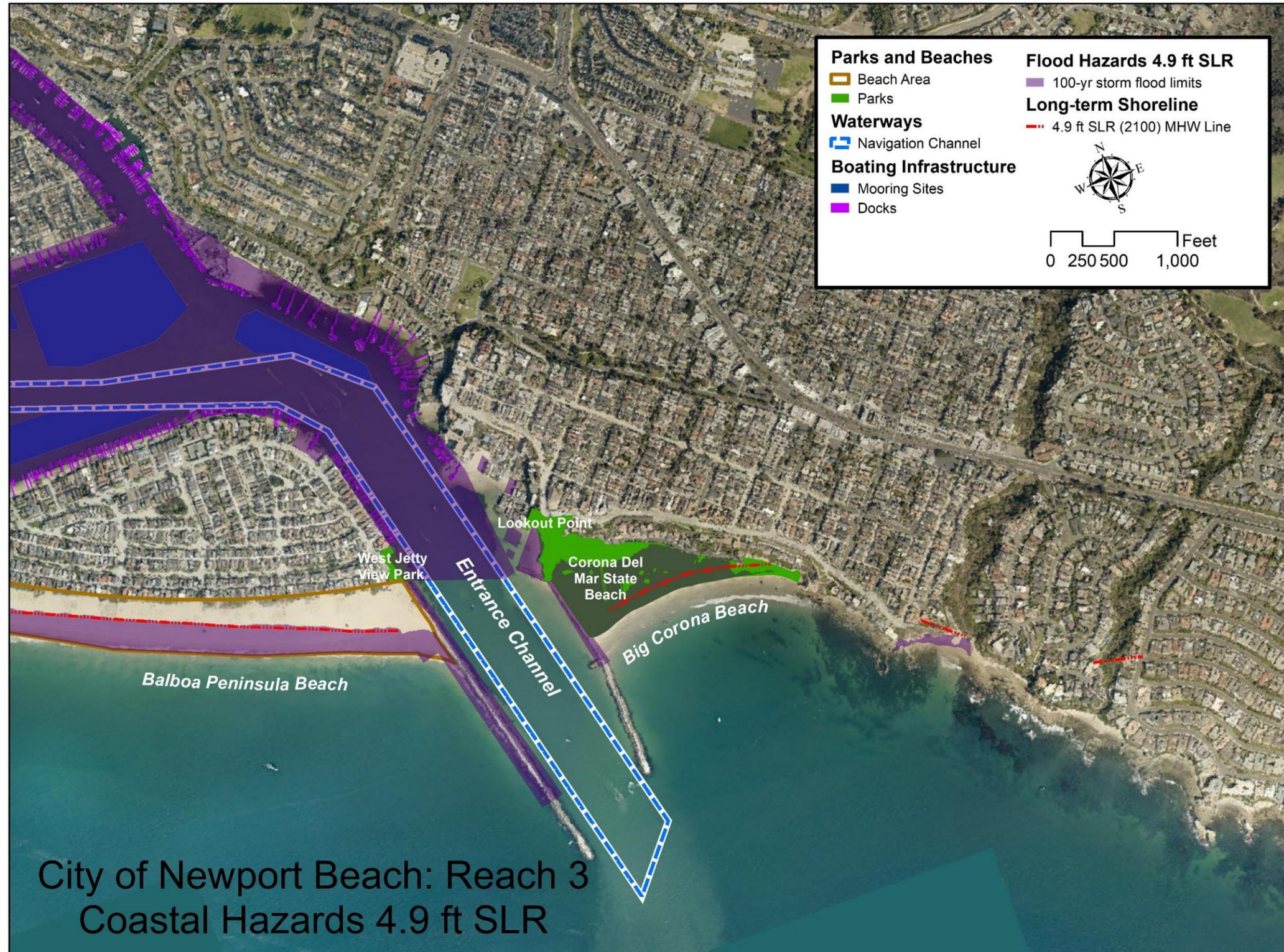
Figure 5-13: Parks, Beaches, Boating Infrastructure, and Submerged Tidelands Assets with 4.9 Feet SLR (Year 2100) Hazards – Reach 3
