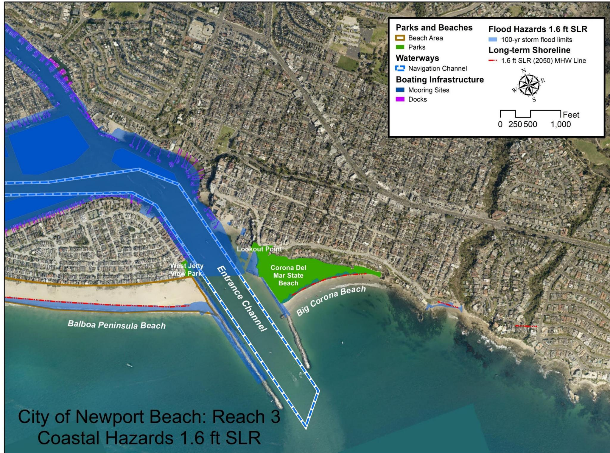
Figure 5-9: Parks, Beaches, Boating Infrastructure, and Submerged Tidelands Assets with 1.6 Feet SLR (Year 2050) Hazards – Reach 3
