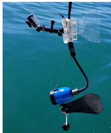
Figure 3. “Splash Cam” underwater camera setup.
