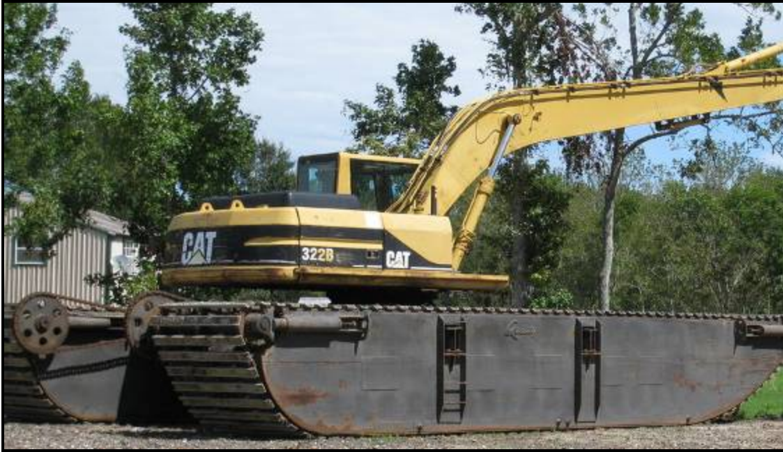
Amphibious Excavator, photo courtesy of DD-M and Cooper's Crane. Amphibious Cat 322BL Long Reach Excavator with: The machine is 34' long, 18' wide, 13' tall and the ground pressure is 2 psi; 60' of reach; 3/4 cubic yard bucket; 5'x5'x31' pontoons
