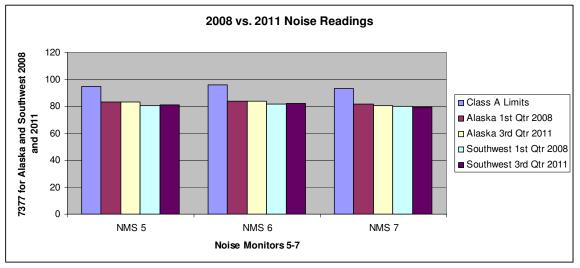
Noise as you may recall from past aviation reports is expressed logarithmically, such that doubling of noise energy results in an increase of 3dB, e.g. 80dB + 80dB = 83dB. An increase of 3dB is barely perceptible to the human ear and an increase of 10dB approximates to a perceived doubling of noise level. This means that a large amount of acoustic energy reduction is required to produce a significant perceptible difference in noise.
