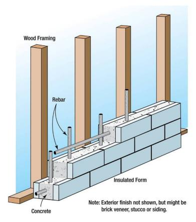
**Figure 6-4. Insulating Concrete Form**
