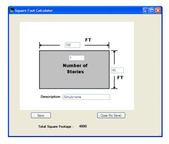
Figure 3-24. Square Foot Calculator Data Entry Screen for Residential Structures
