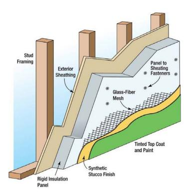
Figure 6-9. Exterior Insulation Finishing System
