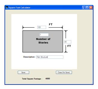
Figure 3-43. Square Foot Calculator Data Entry Screen for Non-Residential Structures
