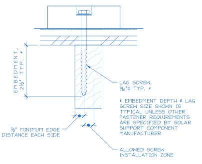
Figure 3. Typical Anchor with Lag Screw Attachment.
