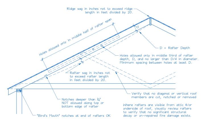
Figure 1. Roof Visual Structural Review (Contractor's Site Audit) of Existing Conditions.
