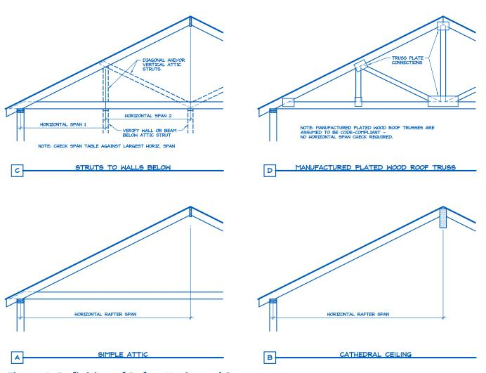
Figure 4. Definition of Rafter Horizontal Span.
