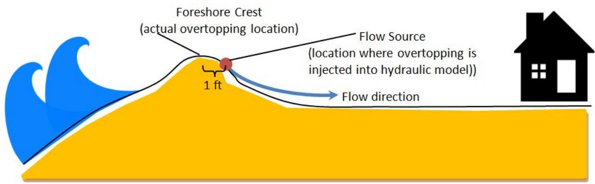
(a) Profile view of injection locations for hydraulic model forcing
