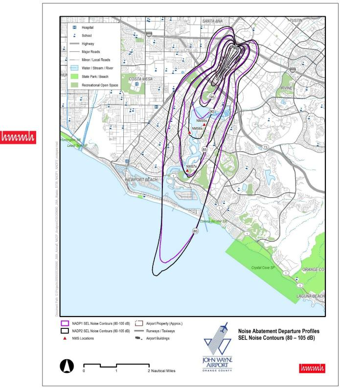
Figure 1. Airline A Boeing 737-800 NADP SEL Contours
