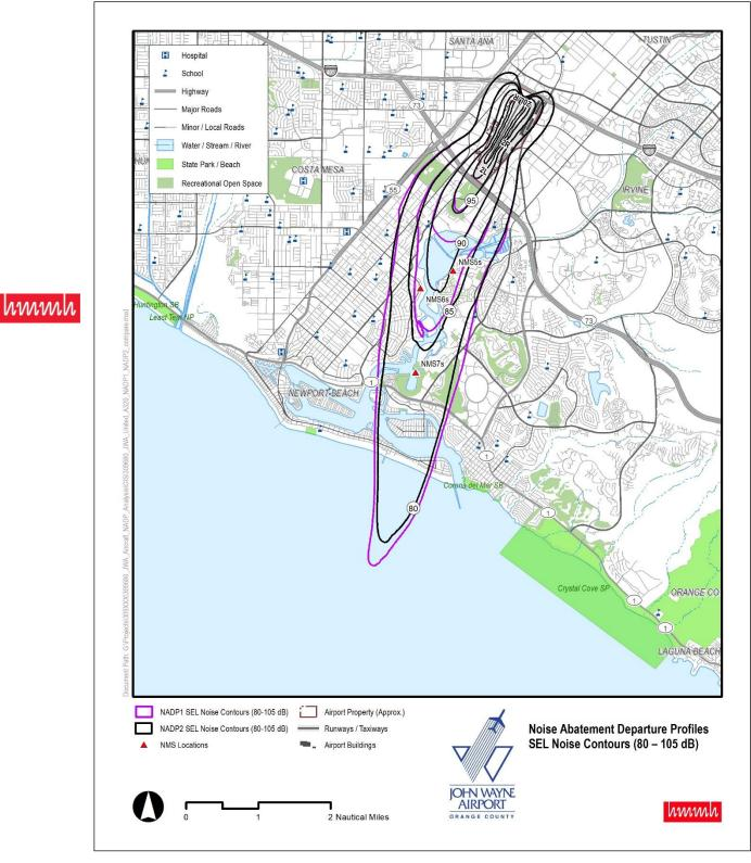
Figure 8. Airline D Airbus A320 NADP SEL Contours
