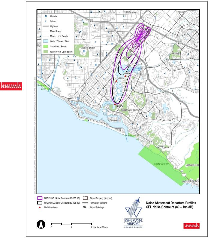
Figure 4. Airline C Boeing 737-800 MAX NADP SEL Contours
