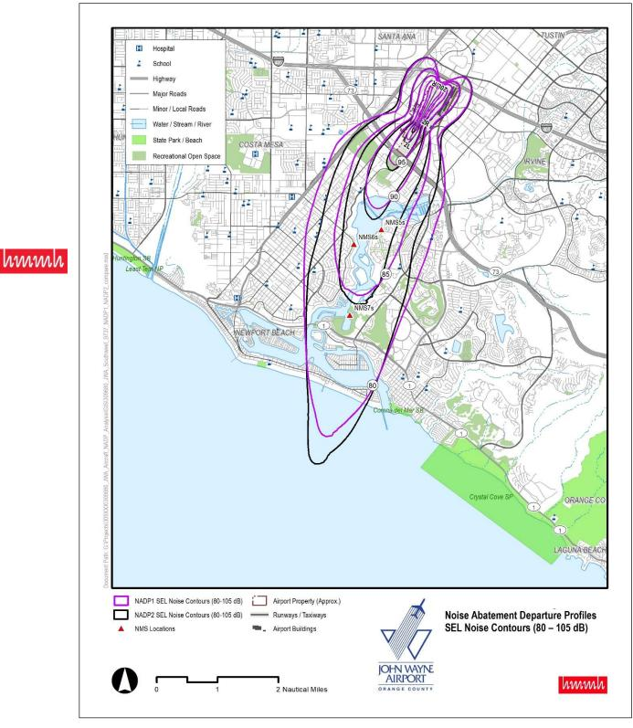
Figure 3. Airline C Boeing 737-700 NADP SEL Contours
