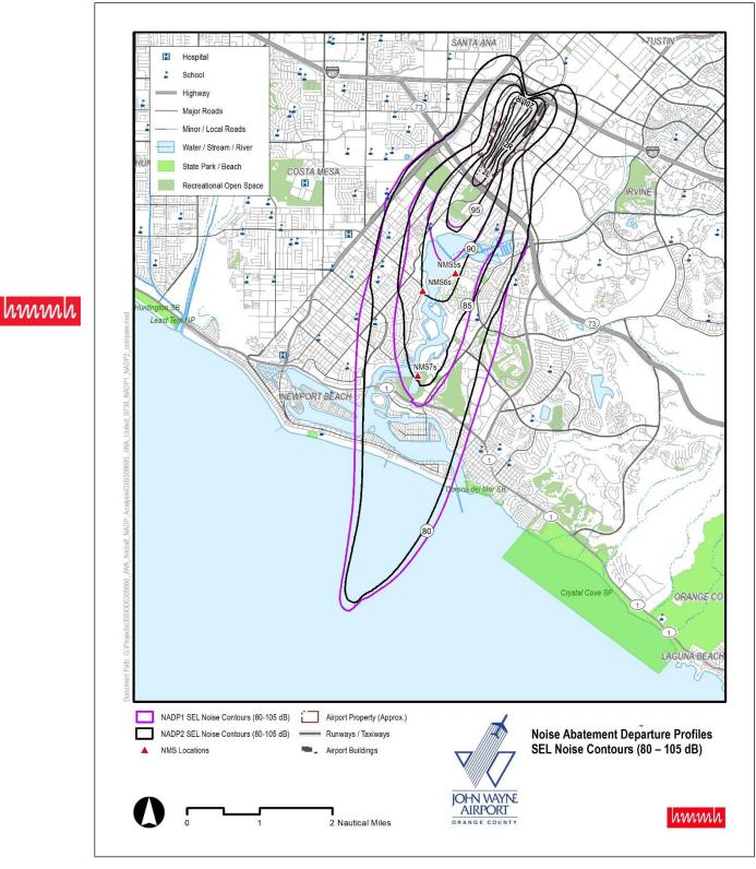
Figure 6. Airline D Boeing 737-800 NADP SEL Contours
