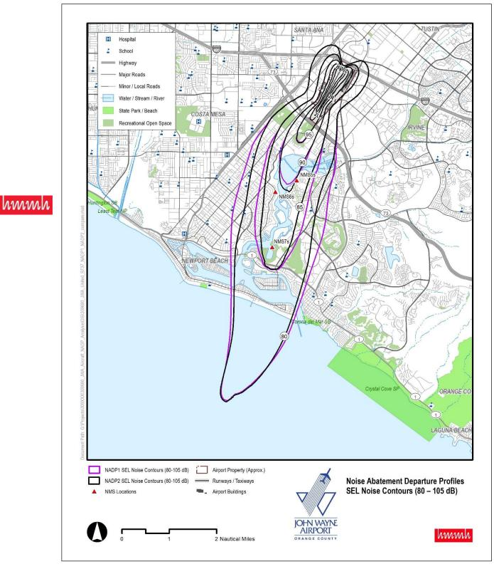
Figure 5. Airline D Boeing 737-700 NADP SEL Contours
