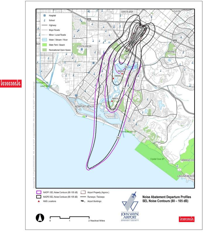
Figure 2. Airline B Boeing 737-800 NADP SEL Contours
