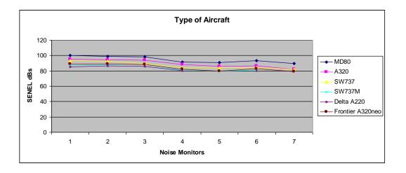
The chart on the following page is a comparison of the old MD80 and the new A220. Just one A220 flight was chosen for comparison. The one flight did not register a noise reading at NMS 5 or 7 and averaged approximately 12.5+ dBs less than the MD80 at the remaining five departure noise monitors. <sup>3</sup>
