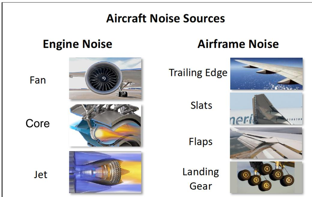
**Fig. 1 Primary Conventional Turbofan Aircraft Noise Sources**
