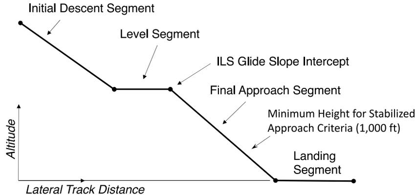
**Fig. 24 Typical Approach Procedure Divided Into Segments**
