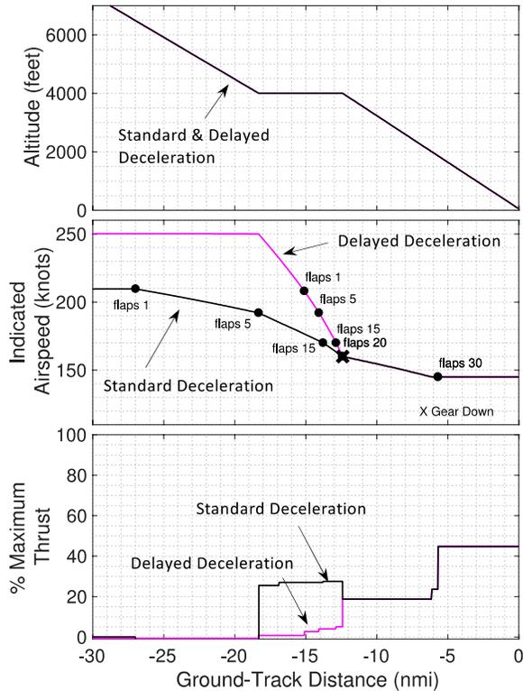
**Fig. 29 Altitude, Velocity, and Thrust Profiles for Representative Wide-Body Aircraft Performing a Standard Indicated Deceleration (black) and Delayed Deceleration (magenta) Approach with 4,000 ft Level-Off**
