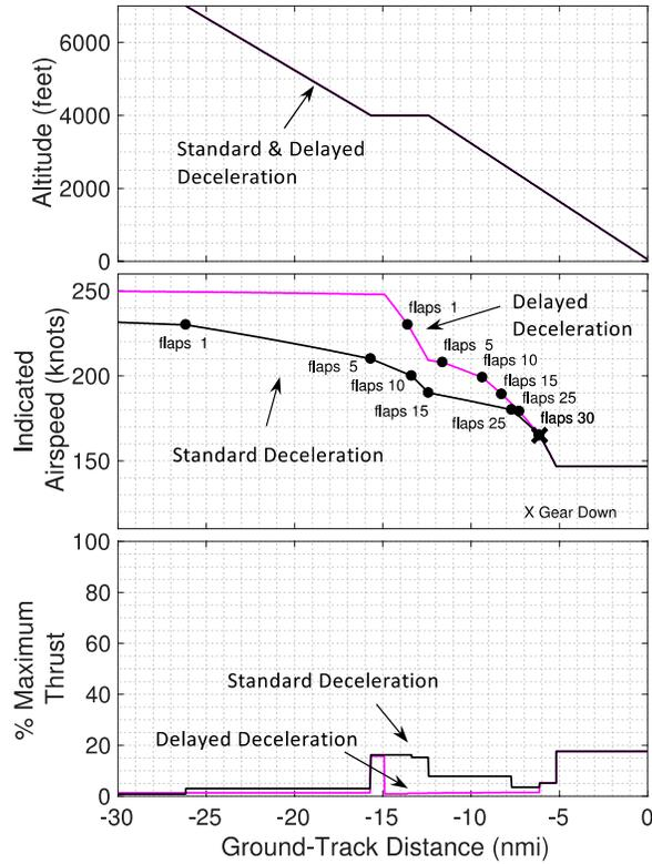
**Fig. 26 Altitude, Velocity, and Thrust Profiles for a Representative Narrow-Body Aircraft Performing Standard Deceleration (black) and Delayed Deceleration (magenta) Approaches with 4,000 ft Level-Off**
