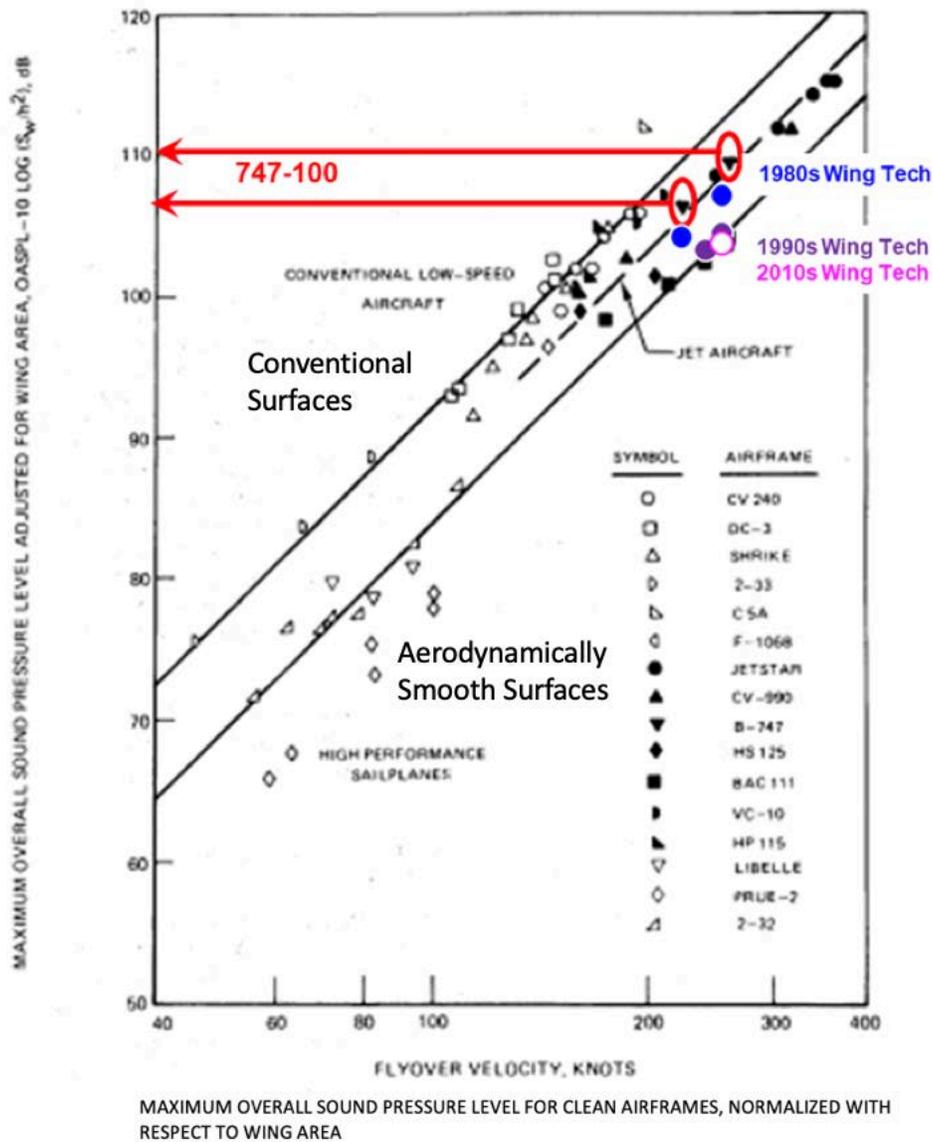
**Fig. 17 Maximum Overall Sound Pressure Level From 1970s flight Fight Tests of Aircraft with Flaps and Gear Up versus Velocity from Ref. [5]. 1980s, 1990s, and 2010s Wing Tech Data Provided by Boeing from Ref. [21]**
