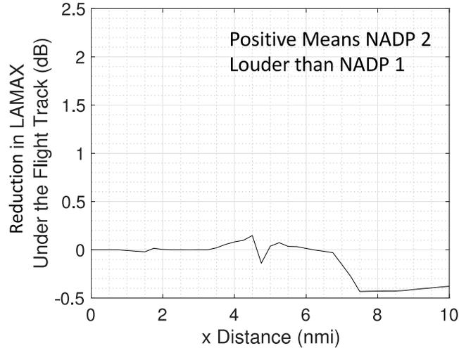
**Fig. 14 Reduction in Undertrack  $L_{A,MAX}$  (dBA), NADP 1 compared to NADP 2 for a Representative Wide-Body Aircraft.**
