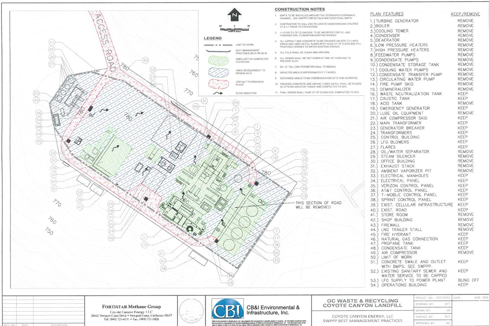
**Figure 5 – Project Site Structures to be Demolished And Structures that will Remain**
