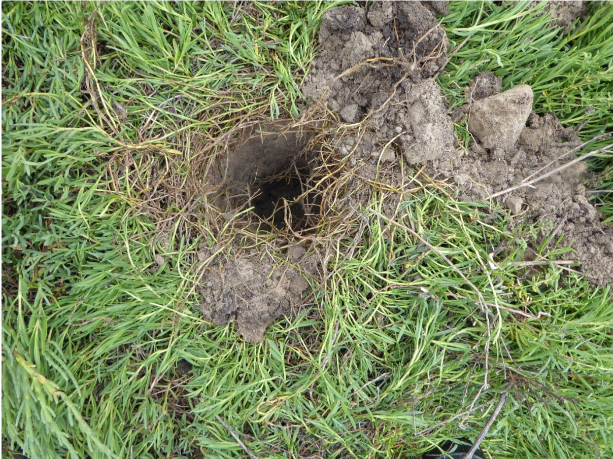
Photo 4 – View of Soil Test Pit No. 2; low chroma soils, sediment deposits, and the presence of wetland vegetation led to the determination that this location occurs within a potentially jurisdictional wetland.
