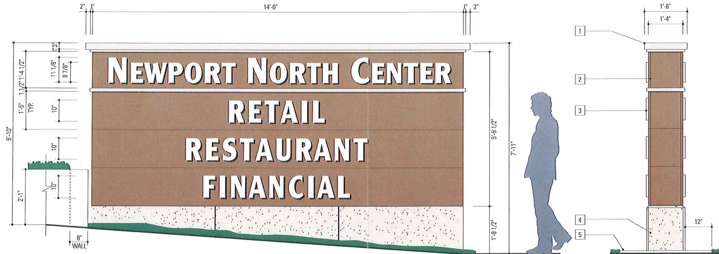
1 ELEVATION - PROJECT/TENANT I.D. MONUMENT SIGN - SIGN NO. 1 - OPTION G (81 SQ. FT. SIGN AREA) SCALE: 1/2" = 1'-0"
