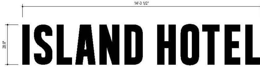
4 ELEVATION - SIGN AT PORTE COCHERE - OPTION 1A (BOLD VERSION OF PROJECT LOGOTYPE) SCALE: 1/2" = 1'-0"
