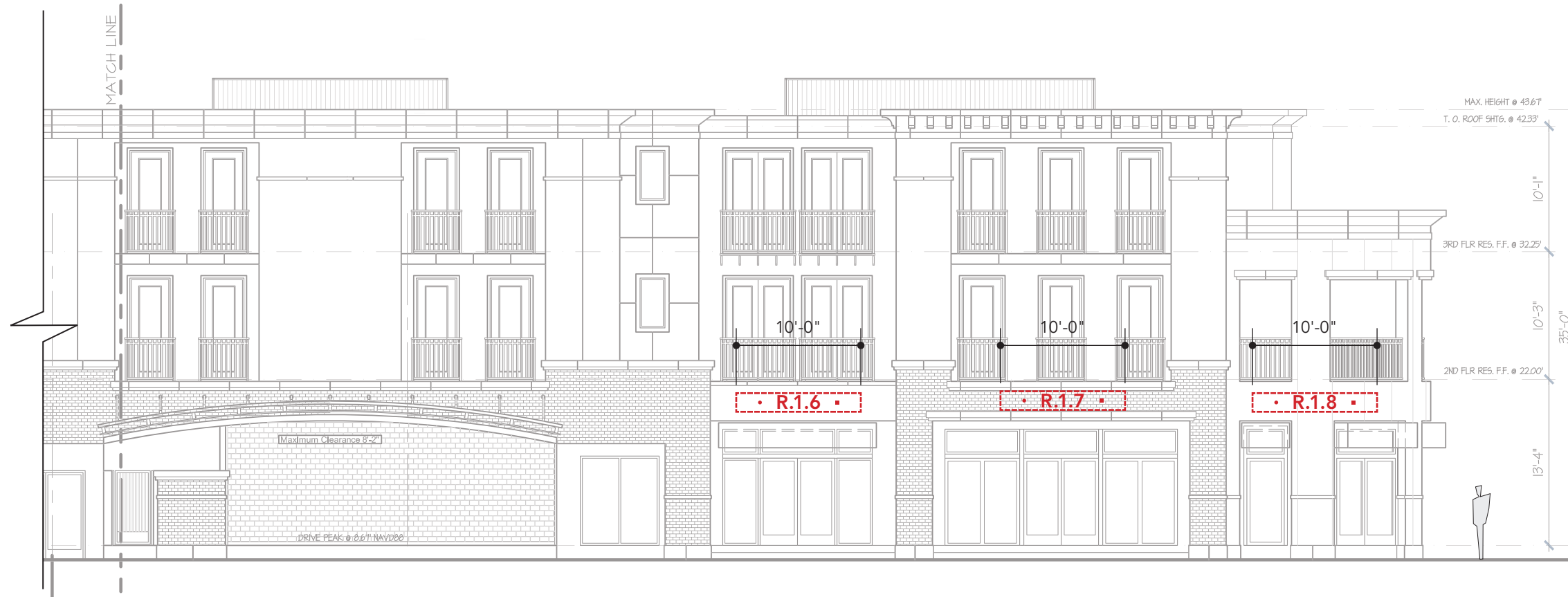
BUILDING A - WEST ELEVATION B SCALE: 3/32" = 1'
