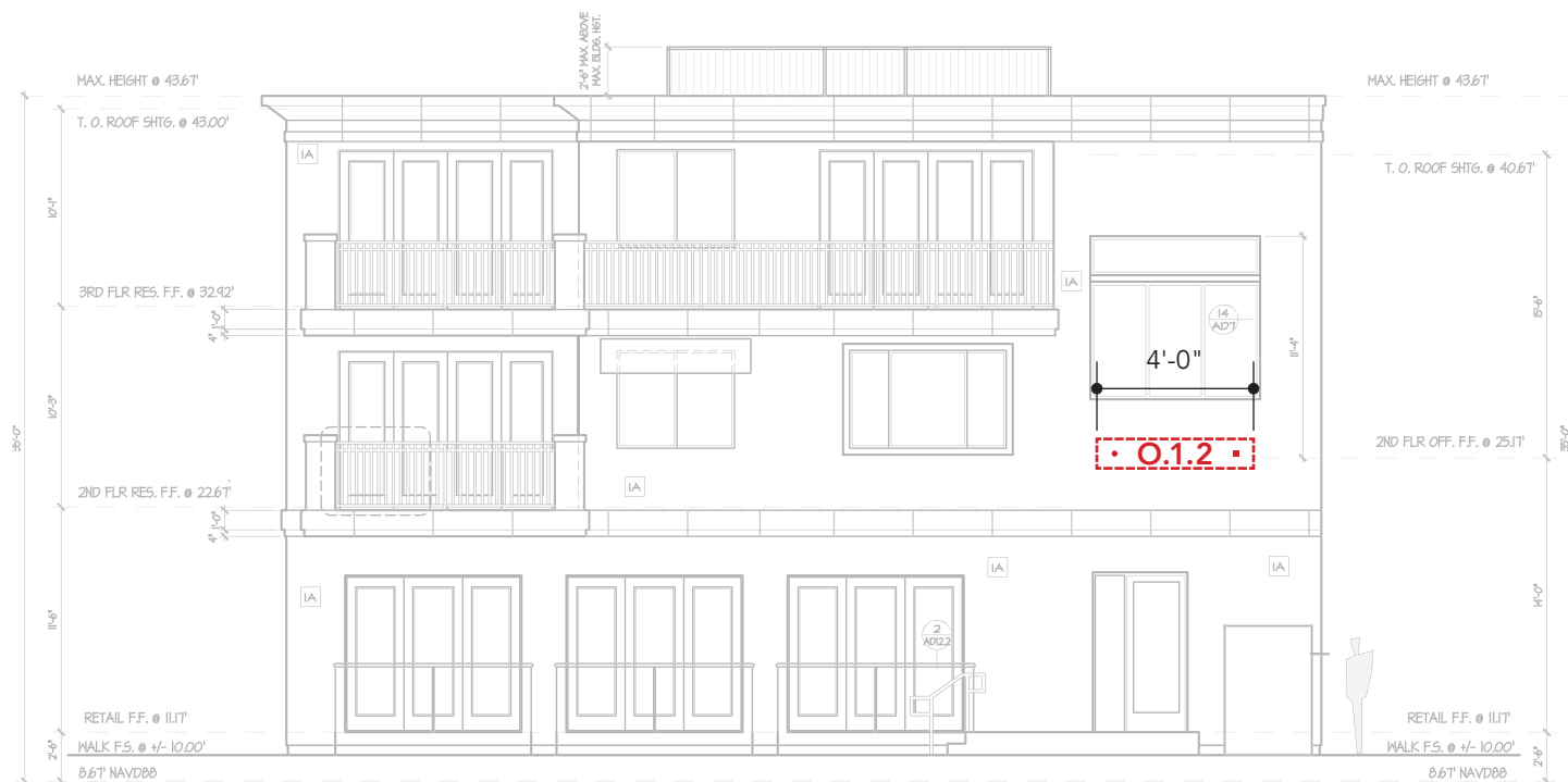
BUILDING H - EAST ELEVATION SCALE: 3/32" = 1'
