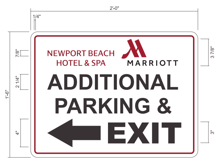
M NON-ILLUMINATED WALL-MOUNTED PARKING SIGN SCALE: 1 1/2" = 1'-0" (QTY. 1) 3 SF GENERAL SPECIFICATIONS: .125" PAINTED ALUMINUM PANEL WITH VINYL COPY APPLIED FIRST SURFACE
