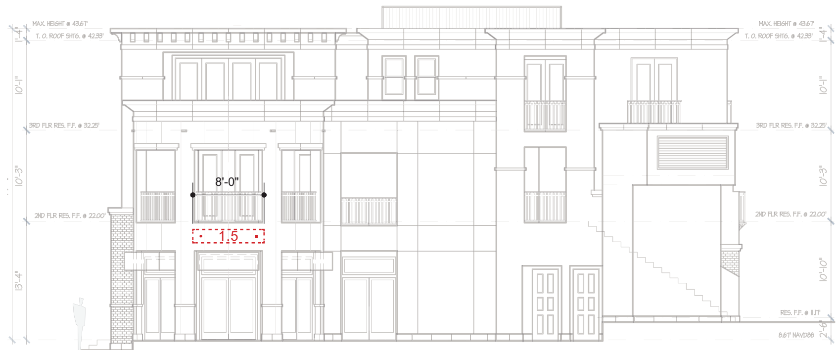
BUILDING A - SOUTH ELEVATION SCALE: 3/32" = 1'
