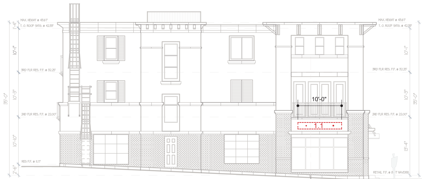
BUILDING A - NORTH ELEVATION SCALE: 3/32" = 1'
