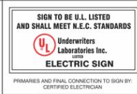
ALL ELECTRICAL COMPONENTS TO BE U.L. LISTED, APPROVED AND MARKED PER N.E.C. 600-4. ALL TO BE ELECTRICALLY GROUNDED PER N.E.C. 250. ALL POWER SUPPLIES TO BE FUSED PER U.L. 48, 20-2.1 GROUNDING AND BONDING PER N.E.C. 250-90, -92, -94, -96. SIGN TO MEET N.E.C. AND U.L. 48 STANDARDS FOR ELECTRICAL SIGNS, GROUNDING & BONDING AS PER N.E.C. 250-90 & NEC 600-7
